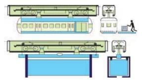
Combination car adapted for automated small container loading on the top left. The vehicle has a movable floor to become a wall allowing automated small freight loading for off peak times gaining extra revenue removing trucks from the roads.
